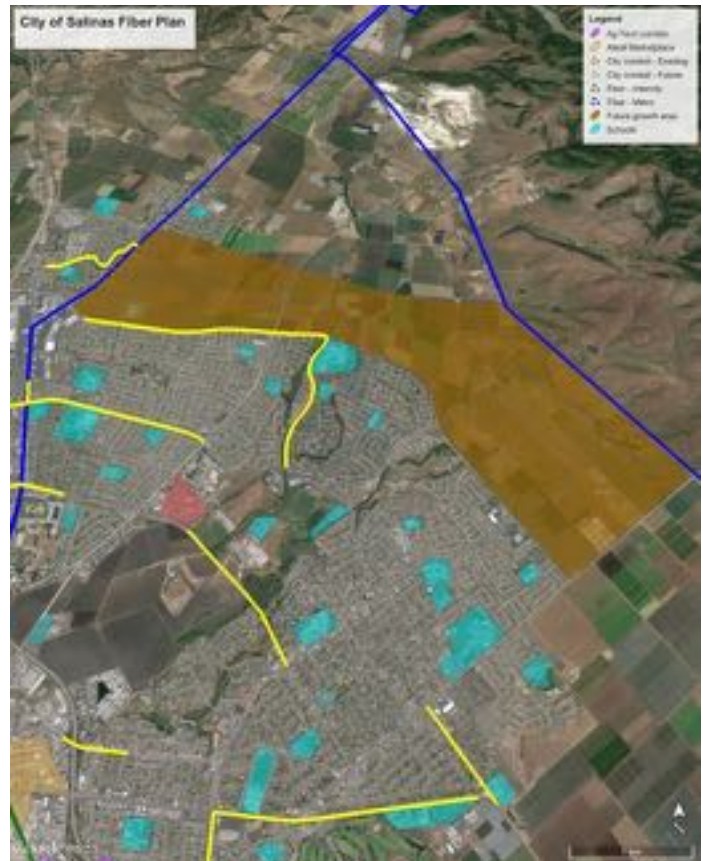
Figure 3.4 – Fiber routes and city-owned conduit in north Salinas.
