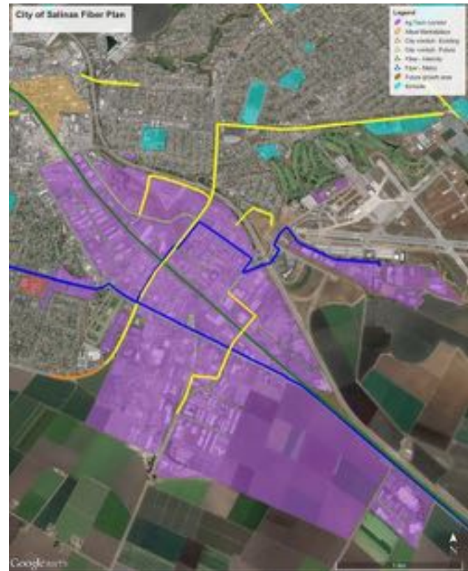
Figure 1.1 – Fiber routes and city-owned conduit in Salinas Agricultural Technology Corridor.
