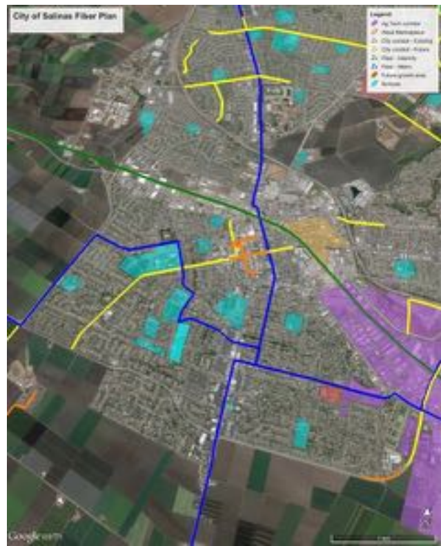
Figure 3.1 – Overview of fiber routes and city-owned conduit in Salinas.
