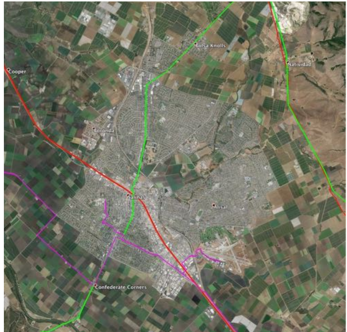
Figure 2.6 – Major intercity and metro fiber routes through Salinas. Purple = Sunesys, green = AT&T & OpticAccess, red = north/south routes along railroad right of way.
