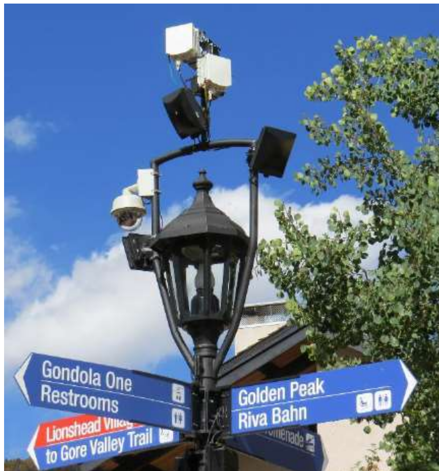
Figure 7 – mmWave Antennas Providing Backhaul for Wi-Fi Network
