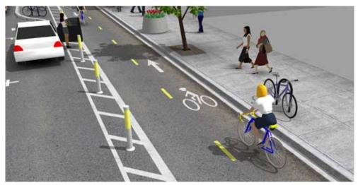
Two way cycle track, separated from the street via bollards. Planters or other decorative elements may be used in place of bollards (Image from NATCO)
