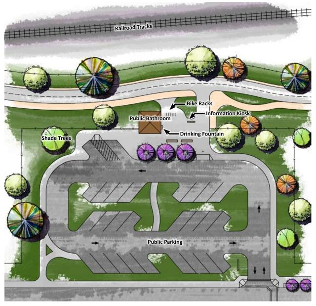
Figure 5-39 Trail Access/Staging Area Design Elements
