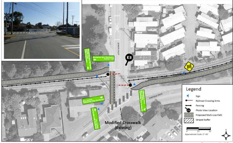
Figure 5-29 Crossing No. 59, 47th Avenue Figure prepared by W-Trans
