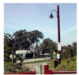
Trail lighting that is dark sky-compliant due to downward-facing light with shield
