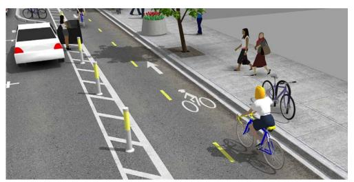
Two-way cycle track, separated from the street via bollards Planters or other decorative elements may be used in place of bollards (Image from NACTO)
