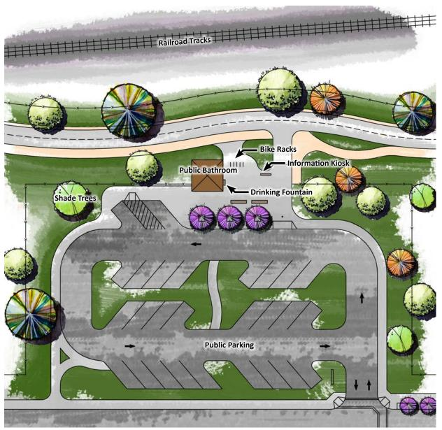
*Figure 5-8 Trail access/staging area design elements*
