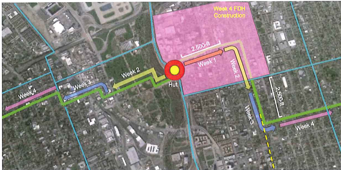
Figure 3-4 - Crew spread between adjacent construction elements, depicting progression of Backbone construction prior to breaking ground on the adjacent FDH.
