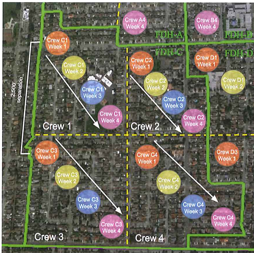
Figure 3-3: Crew distribution and progression methodology within the construction of a single FDH.
