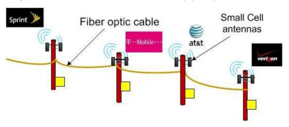
Figure 12 - Illustration of Planned Allocation of Poles to Enable Deployment by Four Wireless Carriers
