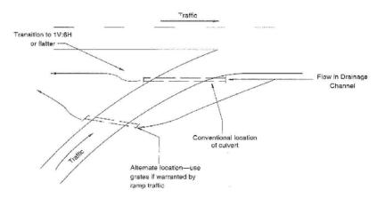
Figure 3-11. Alternate Location for a Parallel Drainage Culvert
