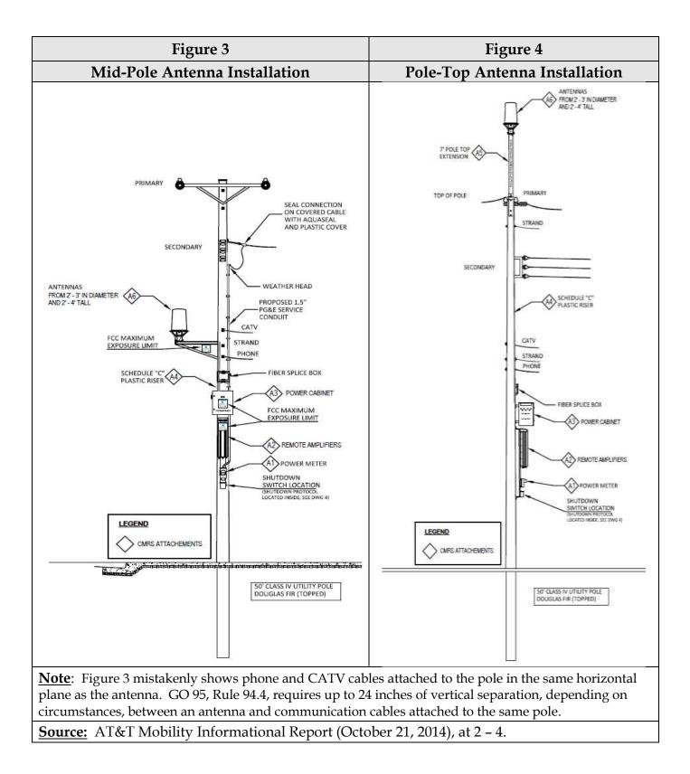
As shown in Figures 1 - 4, above, a typical CMRS pole installation includes an antenna, shut-off switch, power meter, battery backup, radio amplifier, power cabinet, and risers for communication and power cables. The CMRS installation is usually connected to a separately attached communication cable for backhaul.
