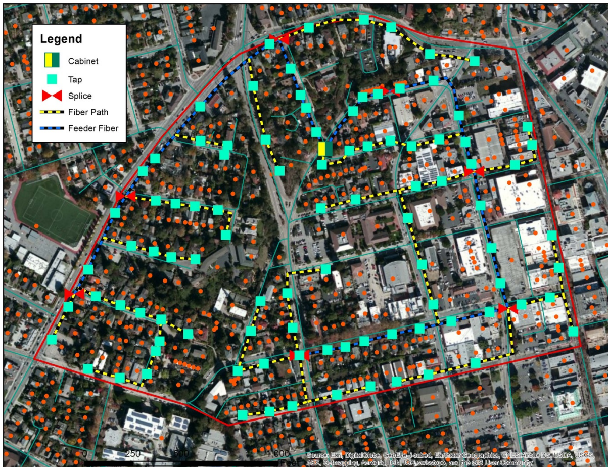
Figure 4: Sample FTTP Access Layer Design
