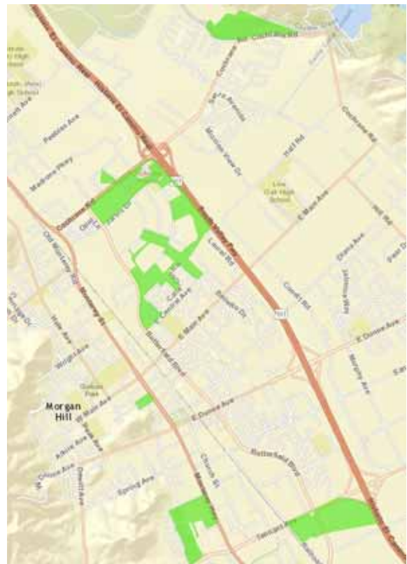
Figure 2.7 – Census blocks with enhanced copper service. Note correlation to commercial and industrial zones. A larger version is in Appendix A.
